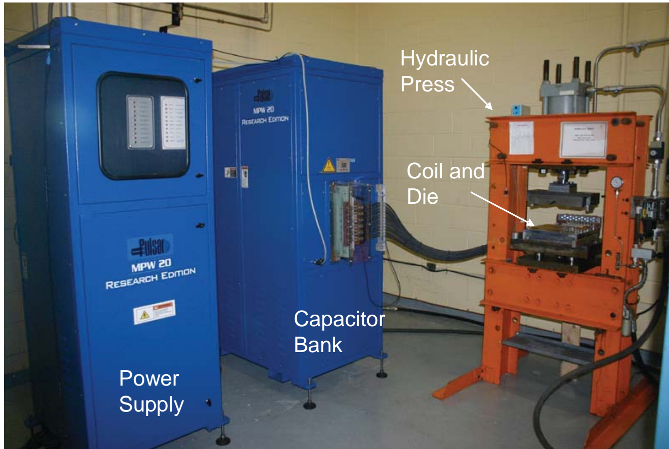
Pulsar Research Edition 20kJ, 9 kV Pulse Generator
