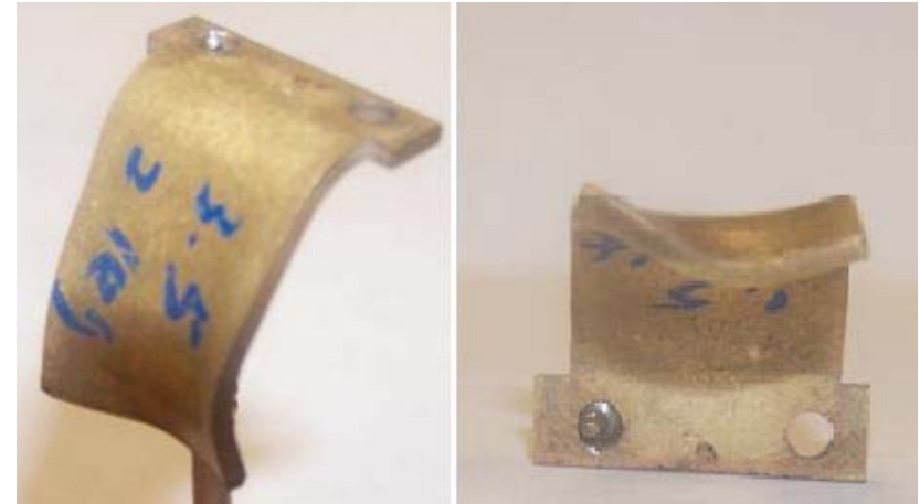
Non uniform flanging of 1.588mm specimen
