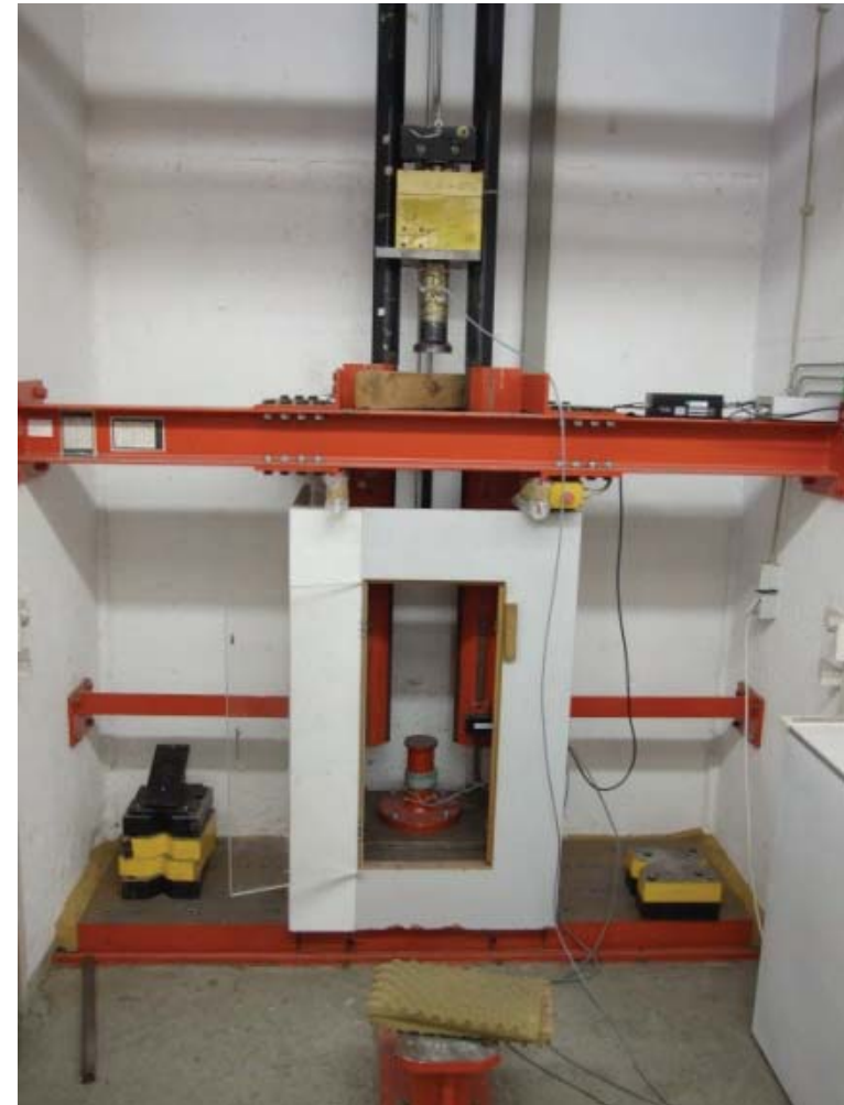
Fig. 3: impact device (left) and drop tower (top)
