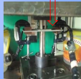
Electric Current input mode in current electro-plastic riveting setup
